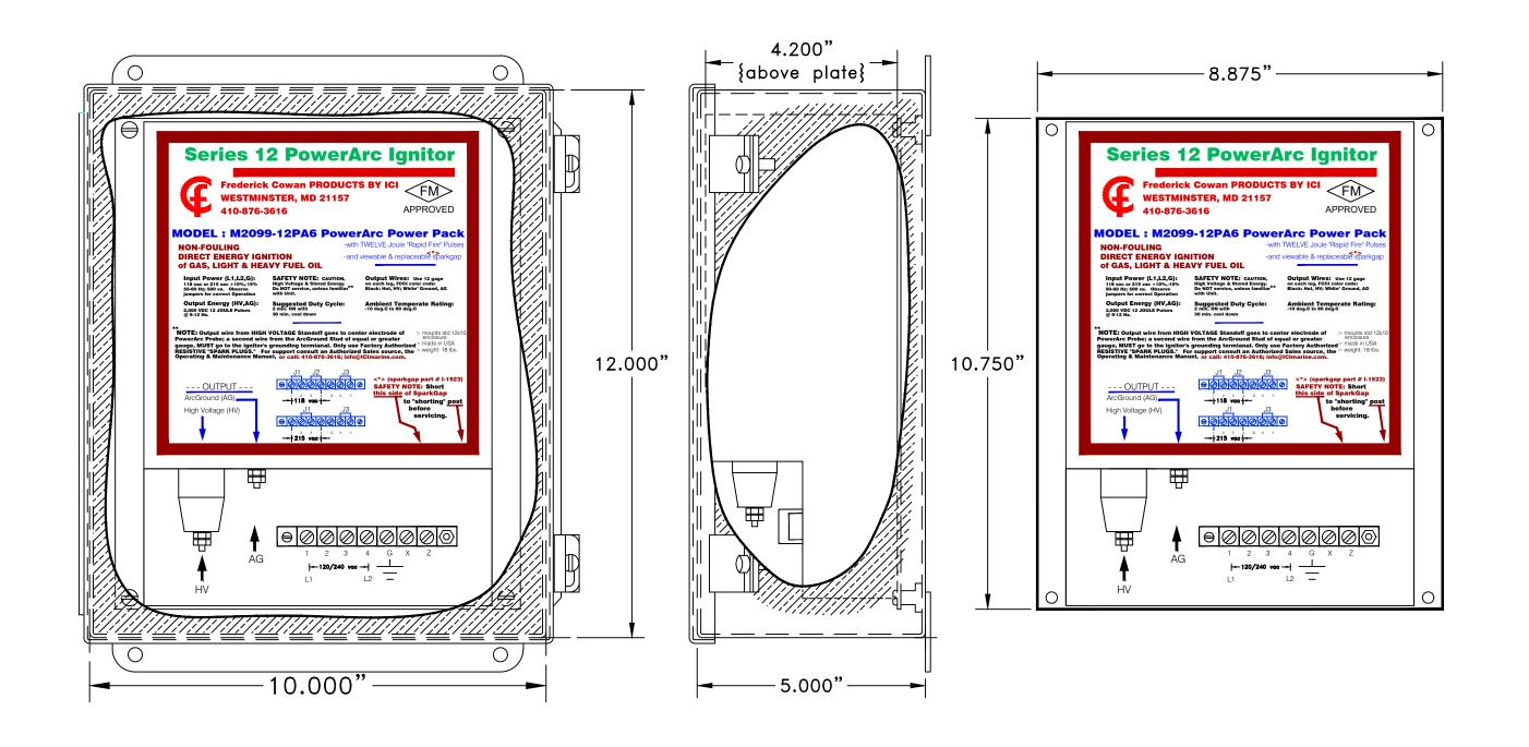
Shown in NEMA 12 Enclosure (M39CA-AF12E-N12) also available NEMA 4, 4XSS, 4XFG, X-PROOF (M39CA-AF12E-N4/4XSS/4XFG/NEXP)
